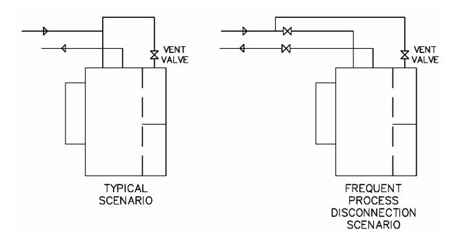
The optimum location for venting is on the top of the overhead return piping above the unit. The customer is encouraged to add an extra vent (Blow-Off) valve at this point. With this new Blow-Off Valve location the return valve and internal blow-off valve should be closed completely during venting. Otherwise air could be pulled into the piping by gravity instead of being removed.
